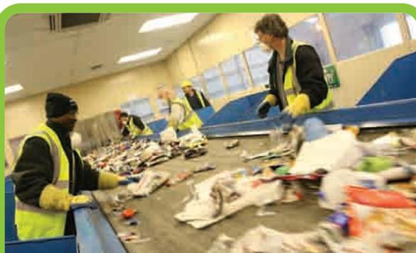
The picking cabin is the final stage in the sorting process.
