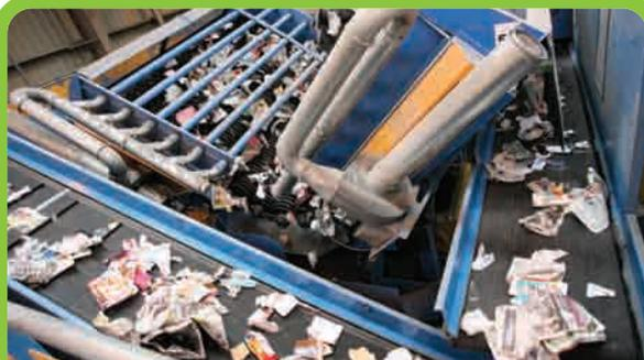
The 'ballistic separator' shakes the materials and smaller items fall through holes onto another conveyor belt.
