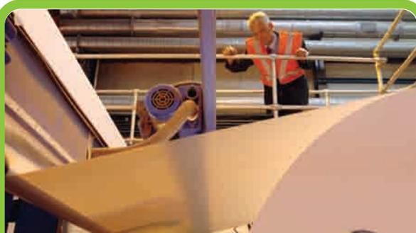
The clean fibres are turned into new paper which is wound onto reels so it can be sold on.
