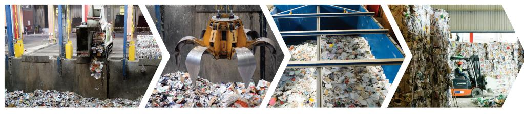
The MRF has a design capacity of 84,000 tonnes per annum and has been designed to process co-mingled materials, delivered loose or in plastic bags, consisting of a mix of one or more of the following dry recyclables: paper, cardboard, glass bottles and jars, clear and coloured PET plastic (e.g. drink bottles), clear and coloured HDPE plastic (e.g. laundry and washing-up liquid bottles) steel and aluminium cans and polycoat material (e.g. Tetra Pak).
