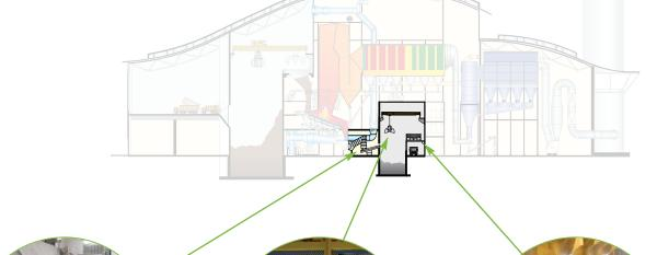
1. The Incinerator Bottom Ash which drops from the grate into a quench bath is then pushed by hydraulic rams onto vibrating conveyors and from there falls into the ash bunker.
