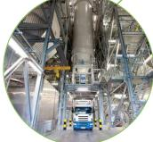
**3.** Compressed air pulses shake off the APCR into silos. The APCR is removed from the site by road tanker.
