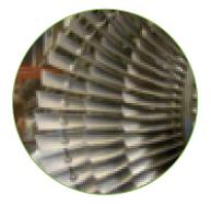
**1.** High pressure steam from each of the three boiler drums is directed onto rings of fixed blades causing the turbine to rotate at high speed.
