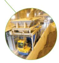
**3.** Incinerator Bottom Ash is discharged from the hoppers into ash containers.
