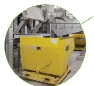
**1.** The Incinerator Bottom Ash which drops from the grate into a quench bath is then pushed by hydraulic rams onto vibrating conveyors and from there falls into the ash bunker.
