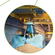
**2.** The Incinerator Bottom Ash is moved by overhead ash cranes from the ash bunker into elevated loading hoppers which are positioned over an internal roadway.
