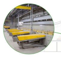
3. The sloping stoker grate consists of alternate rows of fixed and moving cast steel bars. Through the forward movement of these bars the waste tumbles slowly down the burning waste bed. The resulting burnt out product -Incinerator Bottom Ash – falls from the base of the grate
