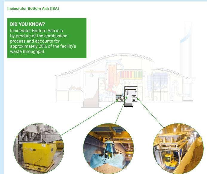
1. The Incinerator Bottom Ash which drops from the grate into a quench bath is then pushed by hydraulic rams onto vibrating conveyors and from there falls into the ash bunker.
