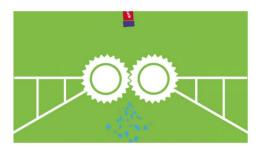
The plastics are then shredded into little pieces or flakes. And then converted into pellets.
