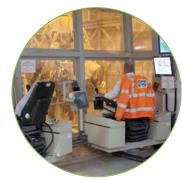
2. Overhead waste cranes mix the waste so it maintains a similar heating value throughout. The waste cranes feed each of the three combustion lines ensuring that each of the boilers has the required feedstock for continuous 24-hour operation.
