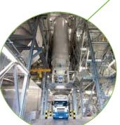
3. Compressed air pulses shake off the APCR into silos. The APCR is removed from the site by road tanker.
