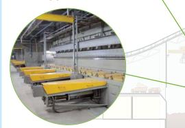
3. The sloping stoker grate consists of alternate rows of fixed and moving cast steel bars. Through the forward movement of these bars the waste tumbles slowly down the burning waste bed. The resulting burnt out product – Incinerator Bottom Ash – falls from the base of the grate into a quench bath.
