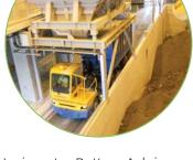
**3.** Incinerator Bottom Ash is discharged from the hoppers into ash containers.
