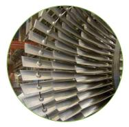
**1.** High pressure steam from each of the three boiler drums is directed onto rings of fixed blades causing the turbine to rotate at high speed.
